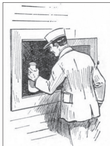
An outer door to the cabinet allowed milk deliveries directly into the cool space.
